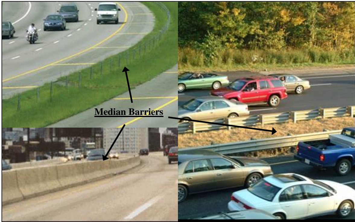
FIGURE 7 Typical Median Barriers(6).
